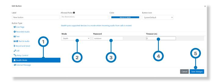
**Stealth Mode** is a feature of some Valcom talkback speakers to provide a listen-only mode when necessary.
