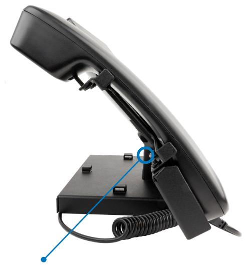
Tilt adjustment for angle of touch screen (located on both sides).
