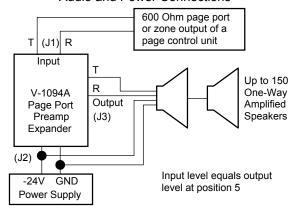
Refer to the figure above for connections. Cabling "D" type station wire or other suitable pairs may be used for audio and power connections.
