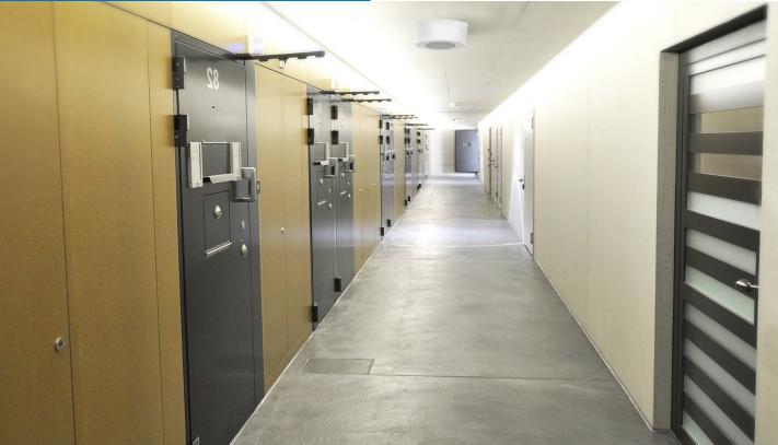
The Valcom Vandal-Resistant Speaker features a steel housing, built-in amplifier, interior security screen and tamper resistant screws. Its smooth, tapered exterior prohibits grasping onto the surface so it stays securely in place. The Vandal-Resistant Speaker is a surface mount design that is ideal for concrete ceilings or any environment where vandalism or damage to the speaker may occur such as correctional institutions, outside entrances and industrial areas.
