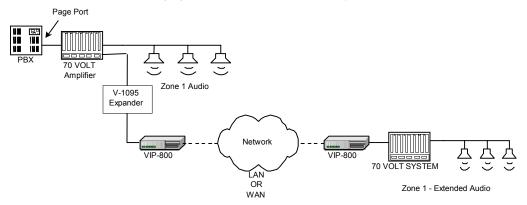
**Note:** During initial SETUP, the "Sub-Net Address" and the "Gateway MAC Number (address) of the Sub-Net Power" **must** be programmed in the software of each unit **locally** - **on the SubNet on which the unit reside**.
