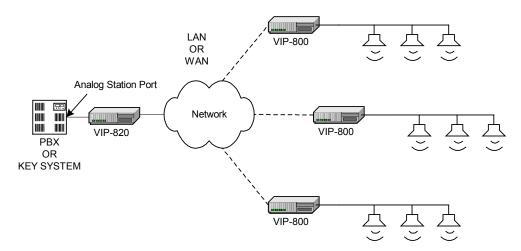
The VIP-820 Networked Trunk Port module makes it a snap to connect two or more PBX systems over the corporate WAN. It provides station to station PBX access, eliminating the need to use expensive trunk connections that are typically required by other competitive products. When the VIP-820 sees an open loop disconnect signal from the PBX Station Port, the VIP-820 will release.
