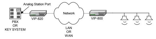
The VIP-820 Networked Trunk Port module can be used to create a multi-zone paging system from one Station Port of a PBX using existing corporate WAN. It provides up to 99 zones with two digit selection. When the VIP-820 sees an open loop disconnect signal from the PBX Station Port, the VIP-820 will release.
