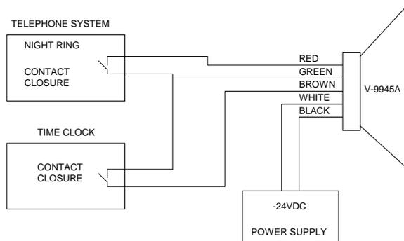
FIGURE 1 - TYPICAL INSTALLATION
